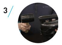
Using a rubber mallet, tap heel until the blade comes out.
