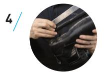
Position the replacement blade where old blade came out, and gently tap it back in with the rubber mallet.
