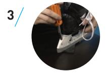
Unscrew the bolt located at the back of the skate to loosen and remove the blade.
