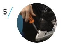
Use the socket with the nut in it, and tighten until it fits snugly (do not over-tighten).
