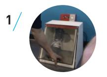
Place skate in heat molding oven at 180 degrees for 12 minutes.
