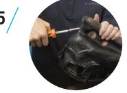
Position bolt back in hole at the back of skate and, using the magnetized socket, tighten bolt into place being careful not to overtighten.
